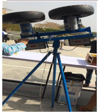
**Fig. 3** – Complete ball projecting machine **Table1** – Speed chart as per motor rpm
