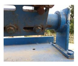
Fig. 2(b) – Mechanism to slide motor plate to vary gap between wheels
